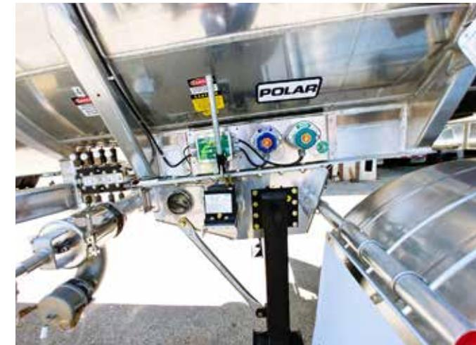
The 2021 Polar trailer, designed and spec’d out for a key customer, also boasts a Scully Load Anywhere Overfill Prevention System.
