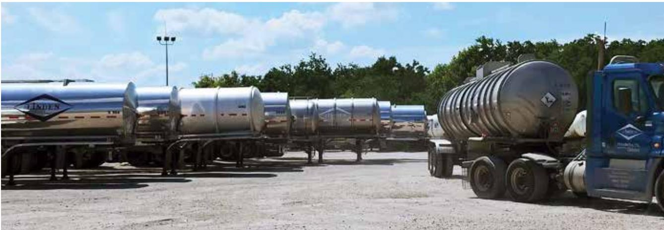
Linden's diverse trailer fleet includes fiberglass reinforced plastic (FRP) tank trailers for bleach and water treatment products, stainless steel and aluminum trailers, compartment trailers, insulated and non-insulated trailers, and center- and rear-loading trailers.
