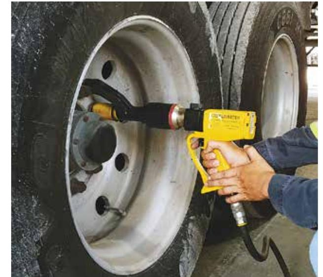
SmartWay-verified Michelin X One wide-base tires, at left, are designed to improve a fleet's bottom line. A Wheelmaster pneumatic torque wrench ensures wheel nuts are safely tightened to manufacturer specifications.
