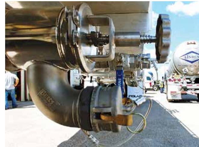
One of Linden’s newest trailers is a custom Polar Tank Trailer with a Betts package of quick-clean valves and Vapor-Pro vapor recovery.
