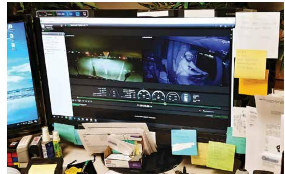
**When an incident is recorded, SmartDrive analysts receive the video, check it for relevancy, score the action, and then send it to Linden Bulk's safety personnel for review.**
