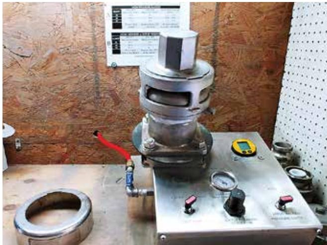
A Pelican Worldwide pressure/vacuum tester ensures Linden's trailer vents are up to code during HM-183 cargo tank inspections.
